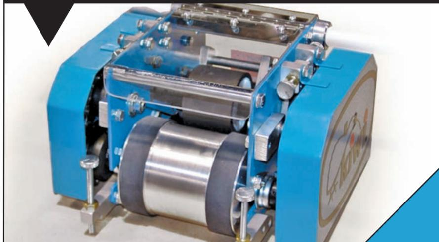
Model 638TI. Table top, hand feed, semi automatic flexo printer for cylindrical parts.
