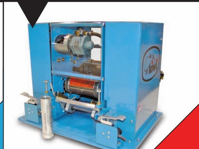
Model 3676TDBHS wide web, high speed capabilities with enclosed doctor blade and web speed matching mounted to flexo base assembly.
